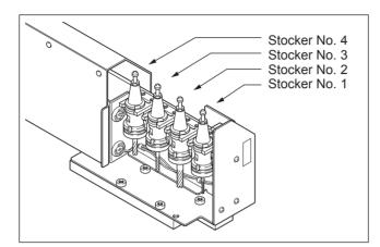
The stockers are numbered from 1 to 4. The tools used for cutting are all specified by these stocker numbers. This makes it important to decide on the numbers where the tool holders are mounted before you perform cutting.
