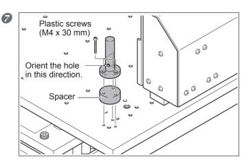
No Rotary Axis Unit Install the Z-origin sensor.
