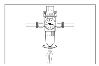
The air regulator is equipped with a filter that becomes filled with trapped material (moisture and dust) over time. Periodically empty the drain. First, stop the supply of compressed air, and loosen the knob at the bottom of the air regulator a little at a time. Material may spray out of the drain at this time. Use a cloth or the like to catch the spray and keep it from scattering. When the drain is emptied, retighten the knob.
