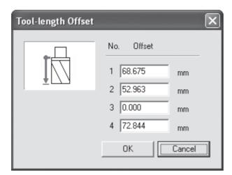
When necessary, you can fine-tune the adjustment values obtained by automatic measurement of tool length. The [Length Offset] dialog box is updated with the results of automatic measurement, so you change the values here.
