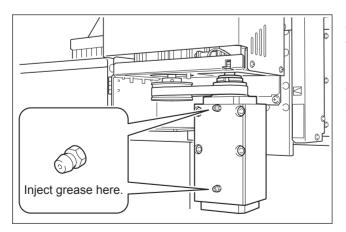
As a general guide, apply grease to the spindle after every 1,000 hours. Inject it using a commercially available grease gun. We recommend using No. 2 lithium grease. Never apply grease containing silicone. Doing so may cause poor switch contact.
