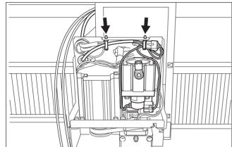
Secure the cabling for the air cylinder in place with retainers.
