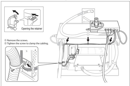
Arrange the cable hose as shown in the figure.
