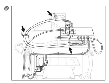
Secure the cable hose in place with large retaining bands.
