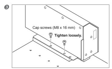
Loosely tighten the magazine unit in place.
