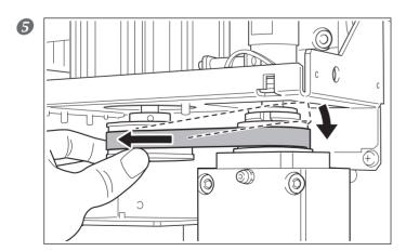
Engage the belt onto the pulley.
