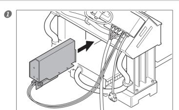
From the rear of the modeling machine, pull in the magazine unit.
