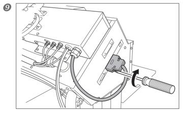
Connect the connector to the modeling machine.
