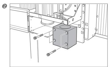
Remove the existing spindle and spindle holder.
