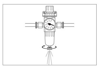
First, stop the supply of compressed air, and loosen the knob at the bottom of the air regulator a little at a time. Material may spray out of the drain at this time. Use a cloth or the like to catch the spray and keep it from scattering. After allowing the air to escape, retighten the knob.
