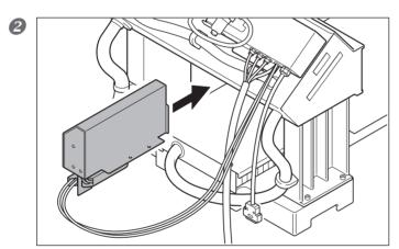
From the rear of the modeling machine, pull in the magazine unit.
