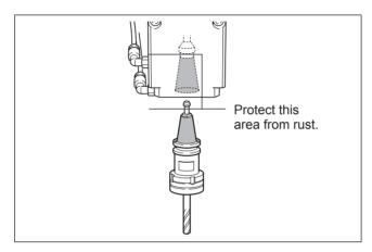
Before use, clean away any cutting waste and excess grease. Failure to do so may affect runout precision or cause slippage.
