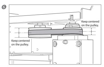
While turning the pulley to break in the belt, keep the belt at the correct position.
